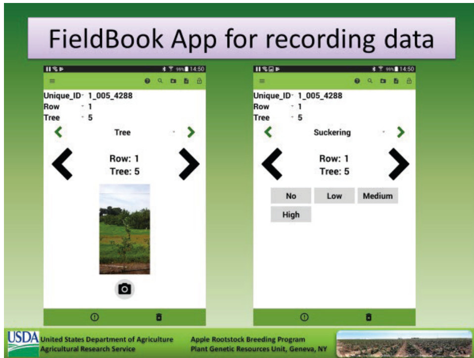
Figure 1. The FieldBook App (available in GooglePlay) is a phenotyping app compatible with most android devices (cell phones and tablets) and allows the collection of visual (properly named images by date, plot and tree number), quantitative, qualitative and voice data that can then be exported for secondary analysis in the form of tables or image files.
