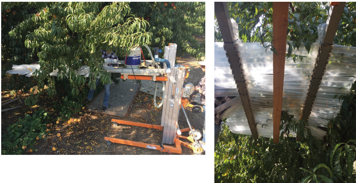
Figure 2 Booms inserted into cling peach tree canopy, as viewed from the side (left) and underneath (right).
